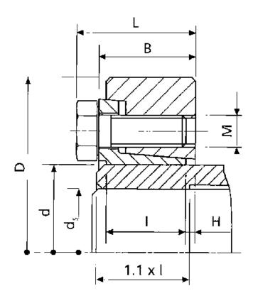
B mm = 31.0 d H8 mm = 75 D mm = 138.0 ds mm = 55 F kN torque = 138 H = 4.0 I mm = 25.0
